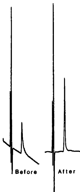
FIGURE 2. Effect of conditioning carbon column on ETU chromatography; 5 ng ETU injected using the HPLC-UV system.
